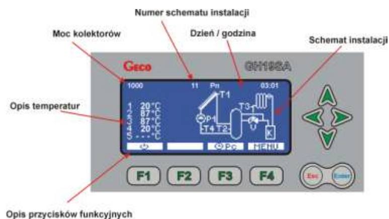
Fig. 3.1. Description of information shown on the display in Auto mode.
