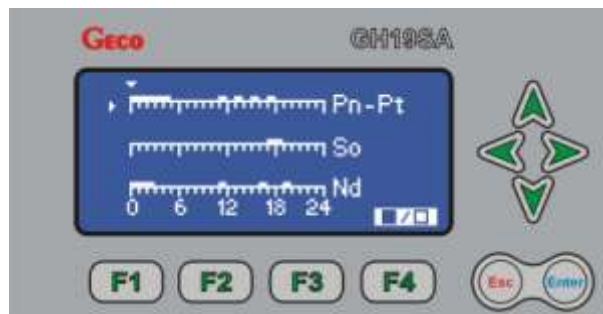
Fig. 3.2. Image shown on the LCD display during operating hours setting for external devices.
