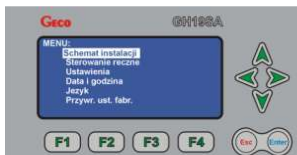
Fig. 3.2. LCD display screen shown after entering the Controller MENU.
