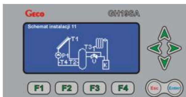
Fig. 4.1. Image shown in the LCD display during selection of the solar collector system diagram configuration.
