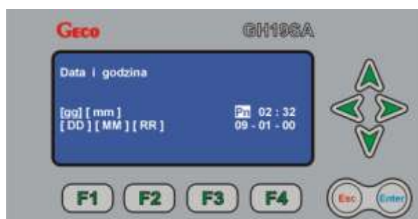
Fig. 4.4. LCD display with date and time setting screen.
