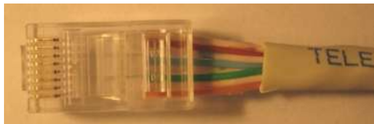
Fig. 2.2. Photo shows termination of the RJ45 connector according to the below description.
