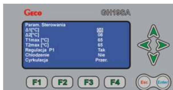
Fig. 4.3. Display screen shown in the control settings editing option. (The setting highlighted for editing on the screen is the \Delta T1 setting)
