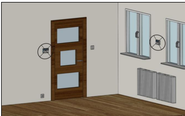
Fig. 1 Examples showing mounting room control panel GA01HA in room.
