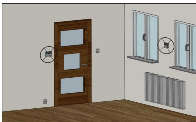
Fig. 1 Examples of correct and incorrect locations for the GA01HC-01 room panel
